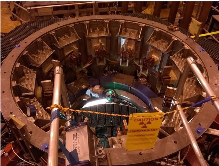
A national laboratory dedicated to research of fusion as a safe and renewable energy alternative has built a tokamak as a research tool. A tokamak is a fusion machine that uses magnets to harness superhot plasma (the 4<sup>th</sup> state of matter) and fuse atoms together, in doing so,
