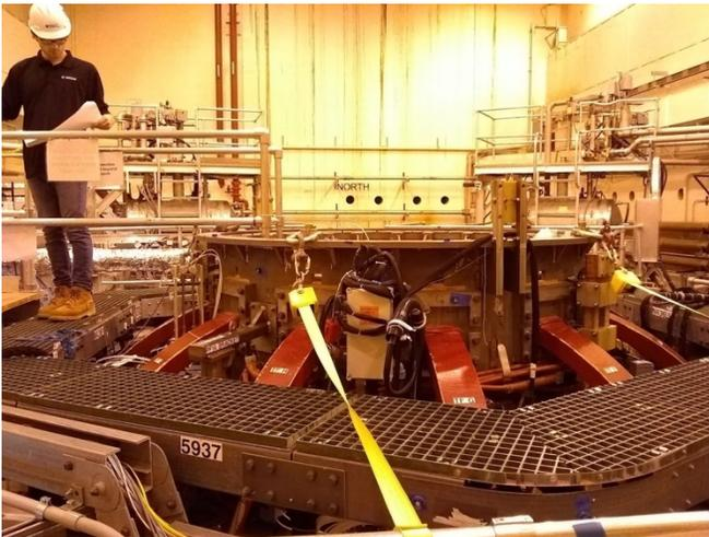
In order to be relative to the tokamak's vacuum vessel, reference features with known locations need to be defined. The reference features to be used are 0.5" and 1.5" SMR control points. When at least three control points are measured, the measuring instrument
