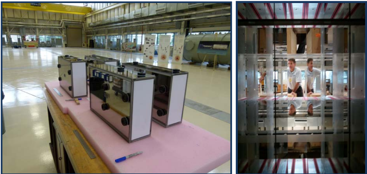
Figure 7 A & B –Glass Beam Segments with Fiducials and Interior View
