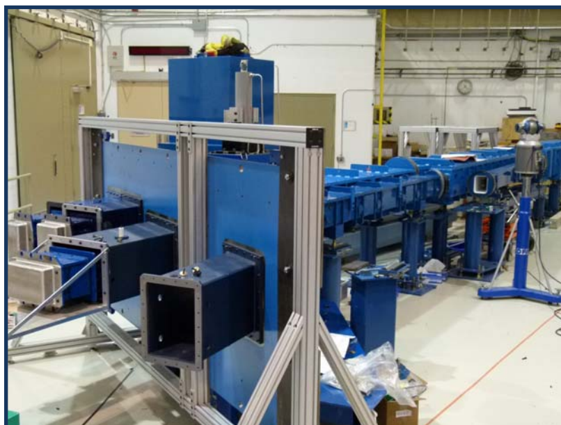
Figure 11 – Assembled Reactor Hall Vacuum Vessels with Wall Penetration Plate
