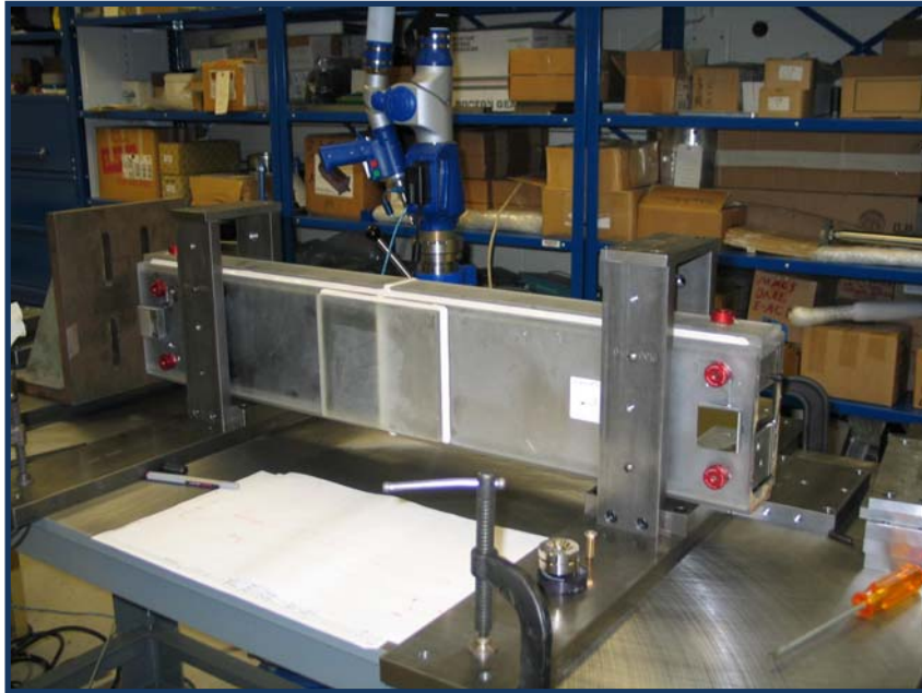
Figure 8 – PCMM Arm Measuring Beam Segment and Fiducials
