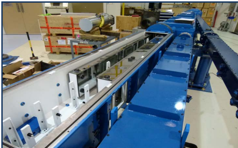
Figure 10 – Beam Segments Installed in Vacuum Vessel
