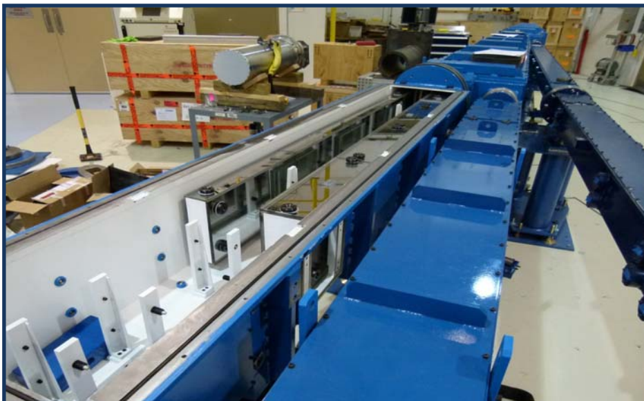
Figure 10 – Beam Segments Installed in Vacuum Vessel
