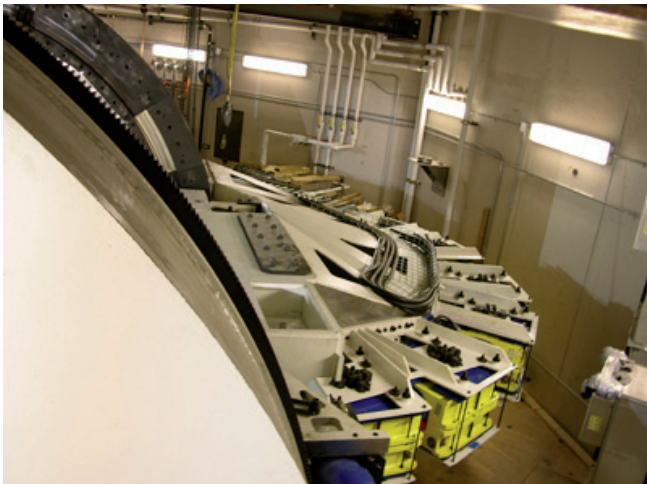
Proton beams are delivered through the gantry and nozzle to isocenter.
