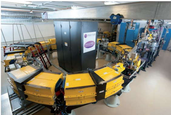
Synchrotron (proton particle accelerator)
