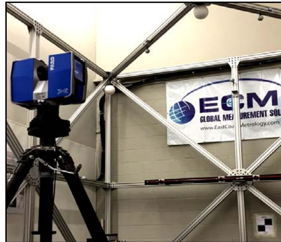
Figure 3: Faro Focus x330 shown with common scanner targets.
