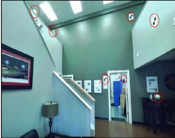
Figure 4: Scanner photograph of a master scan location, with targets circled in red.
